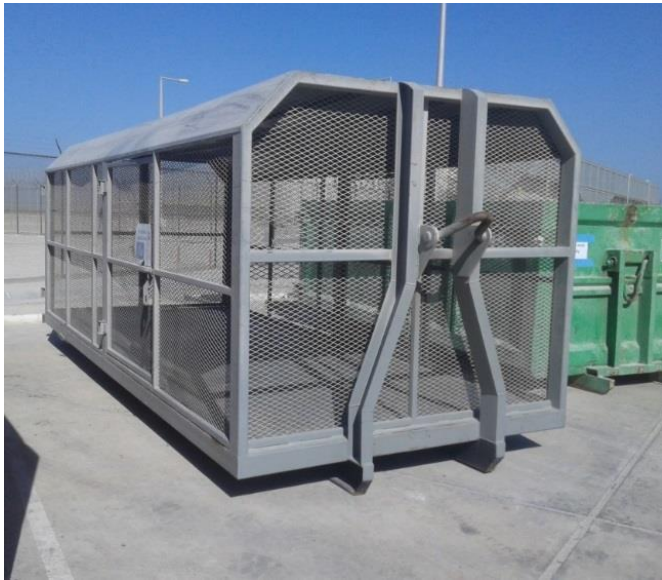
The above picture shows the truck mountable cage for plastic recycling with a hook for easy removal by a skip loader truck. Plastic is deposited into the cage and the door is always kept closed to avoid materials from flying out.
