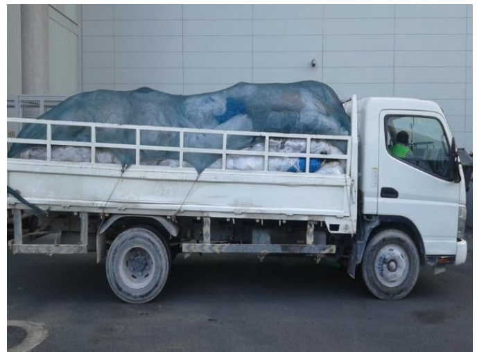
The capacity of the truck is very limited. Extra manpower was spent to fix the net for covering the waste for each trip. The plastic waste would be blown away by wind creating FODs during transportation.
