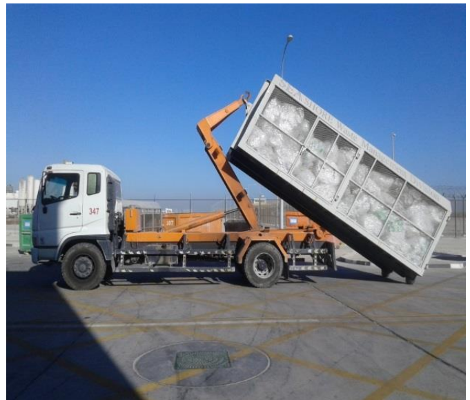
When the cage is full, the truck will bring an empty cage for replacement without extra manpower for transferring the waste from the cage to the truck. The capacity of transportation is doubled compared to the previous truck.
