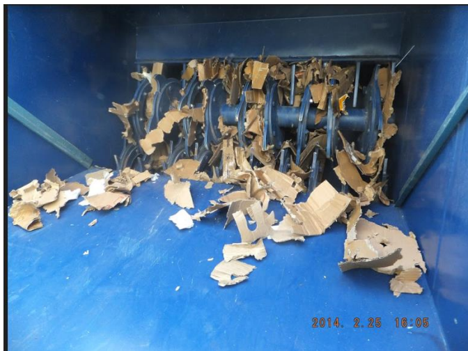
Shredding process for the paper waste that supports the minimization of the waste generated by the terminal activities
